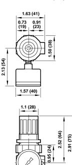
Panel mounting hole diameter 1.19" (30 mm) Maximum panel thickness 0.25" (6 mm)
