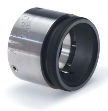
The AST 60 is a simple and easily installed seal that can be used wherever a highly reliable, anti-clog seal is needed. Its narrow seal face design and hydraulic balance make it a cool-running seal. The floating rotary seal ring eliminates seal face distortion inherent to shrink fit designs. Since all the springs are isolated from the pumped fluid, flush rates can be reduced to minimize product dilution.
